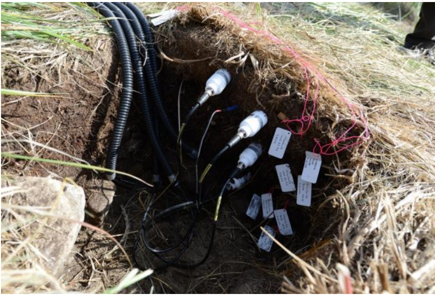
Fig. 5. T1 at Iffiartarfik with the installed sensors and modern bone and wood samples.
