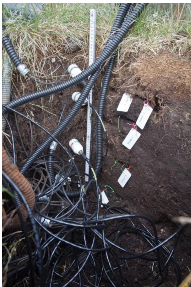
Fig. 3. Modern wood and bone samples installed in the profile of hole 6 at Kangeq.
