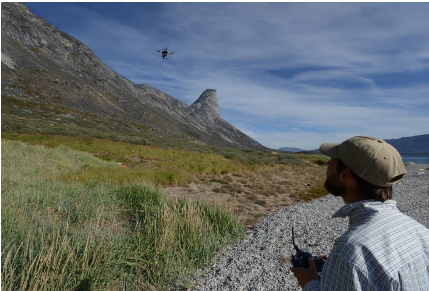
Fig. 6. A quadcopter UAV (Tarot 650-sport) was used to conduct a mapping survey at Iffiartarfik.
