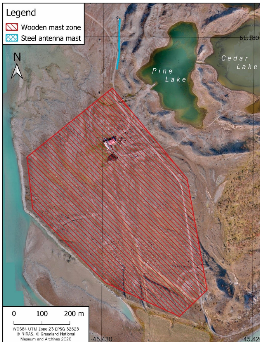
Fig. 113. The wooden mast zone at Camp Corbett covered an area of approximately 31 ha. During the station's operation over 50 wooden masts would have comprised the high-frequency antenna array. The remains of the 185 m steel mast antenna lies directly north of the wooden mast zone.
