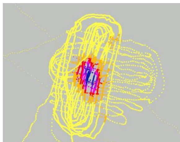
Figure 60: a) Profile showing the intensity of the magnetic field along a profile mapped at Site B on Meteorite Island. b) Color coded magnetic field measurements at the same location as a). The field strength increases from 56000 nt (Yellow) to 61000 (dark blue)
