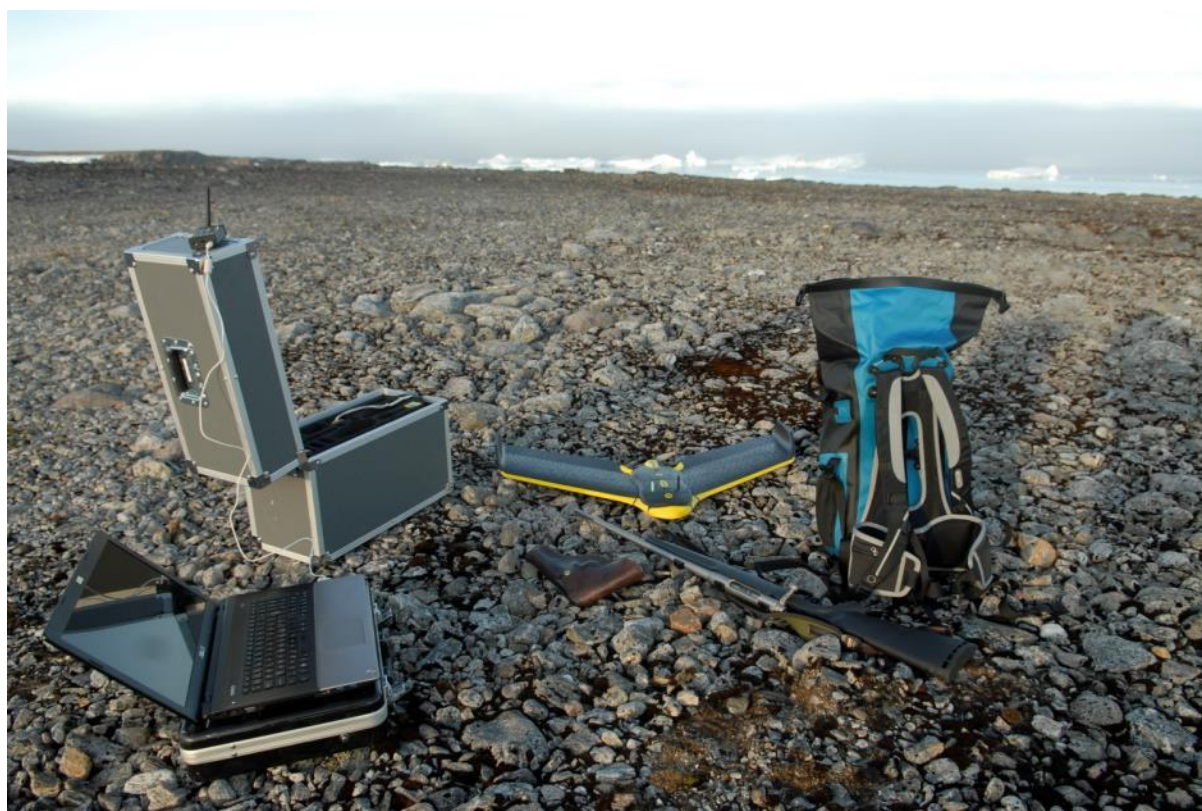
Figure 63: As seen on the photograph the UAS equipment does not take up much space. The fixed-wing Styrofoam drone itself weighs less than 700 grams. Terrain obviously has to be taken into consideration when planning landing spot. Mikkel Myrup del.
