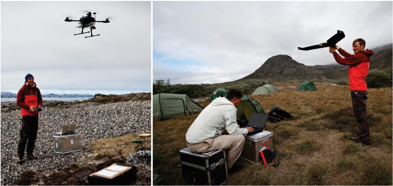
Fig. 2. Left: Fenger-Nielsen piloting the Tarot 650-aport Quadcopter at Ersaa. Right: Myrup and Fenger-Nielsen programming the flight path of the eBee at Sandnæs (photos: Fortuna 2016, Danish National Museum).
