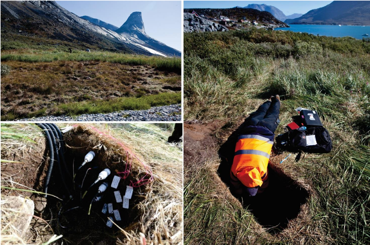
Fig. 6. Archaeological testing at Iffiartarfik. After the archaeological testing was complete in T1, data-logging equipment was installed and modern bone and wood samples were embedded in the wall of the trench prior to backfilling.
