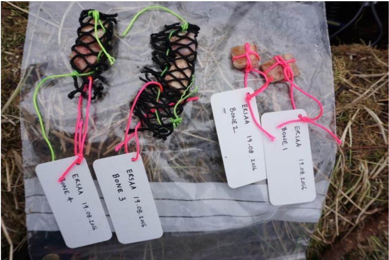
Fig. 9. Prior to installation into the walls of test trenches, bone samples were sewed into fishing net as triplicates or secured with a string attracted to the numbers.
